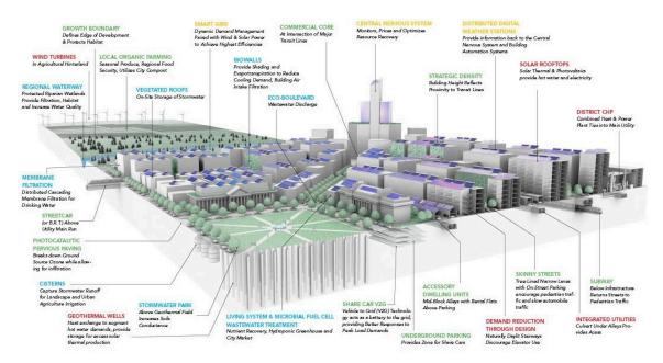
**Figure 16**: An architectural rendering of a sustainable urban district. Features labeled in green are part of the land use and mobility cycle; in red are features of the energy cycle; in blue are features of the water cycles; and in yellow are features of the information cycle.<sup>41</sup>
