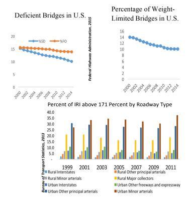
About 10 percent of highway bridges have been posted – having legally reduced load limits due to their condition. Pavement condition on Interstate highways is better than on lesser roads, with more heavily used urban facilities showing deterioration.
