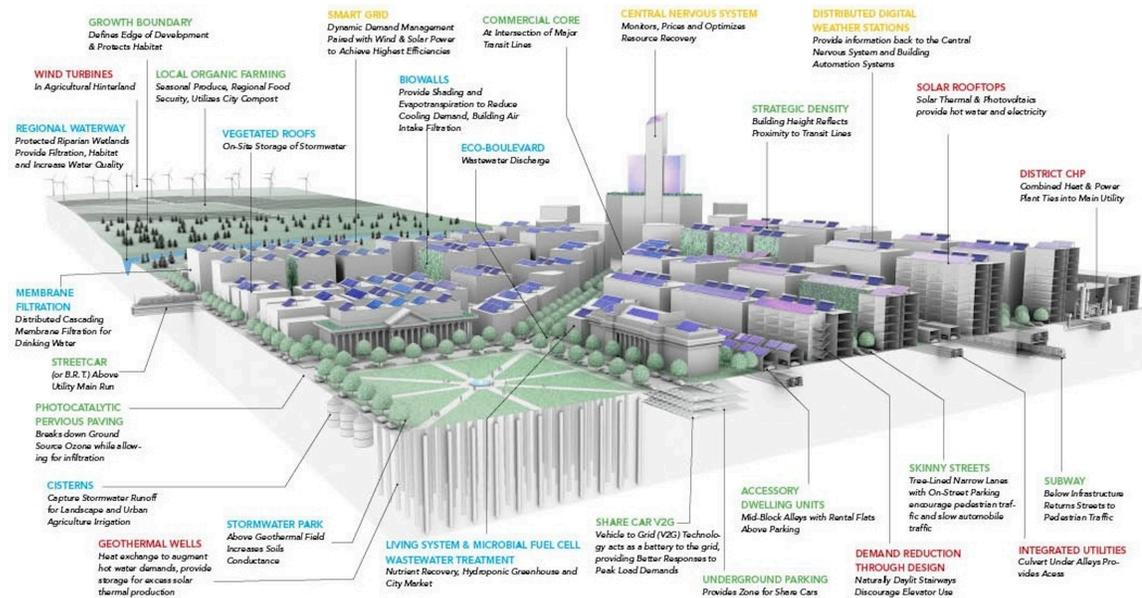
**Figure 16:** An architectural rendering of a sustainable urban district. Features labeled in green are part of the land use and mobility cycle; in red are features of the energy cycle; in blue are features of the water cycles; and in yellow are features of the information cycle.<sup>41</sup>
