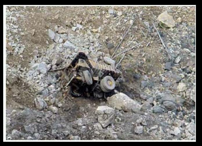
A haul truck driver was seriously injured when he lost control of the truck while hauling overburden to the dump area. The driver was traveling at an excessive speed and the loaded truck veered left into soft material and through the berm on the edge of the dump. The truck overturned and rolled 525 feet on a 38 degree slope. The driver was wearing his seatbelt and the truck was equipped with a ROPS that saved his life.
