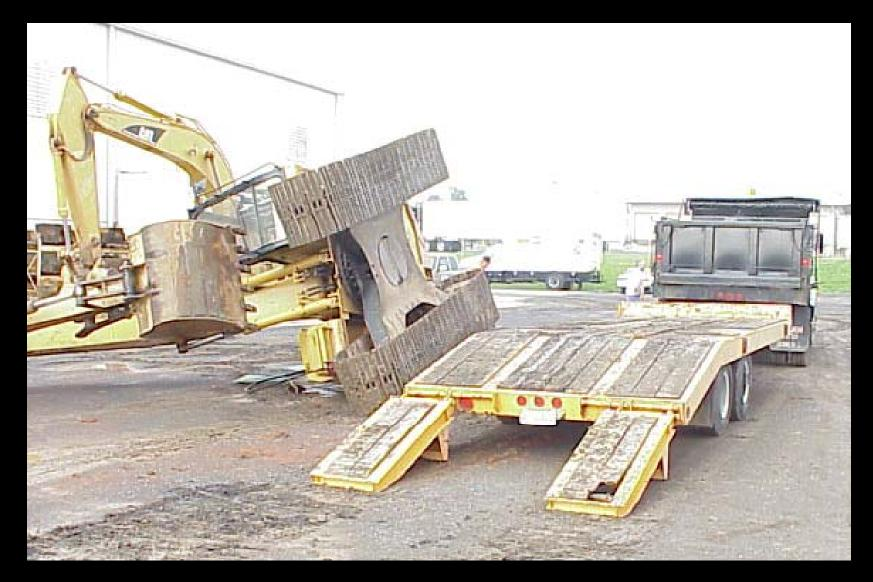
Loading and off-loading equipment can be hazardous. Always wear your seat belt.
