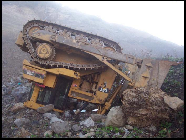
(ROPS) are designed to provide protection to an operator in the protected space of the cab. Your seat belt is a critical part of the Rollover Protection system. Using your seat belt assures your safety when the ROPS is needed.
