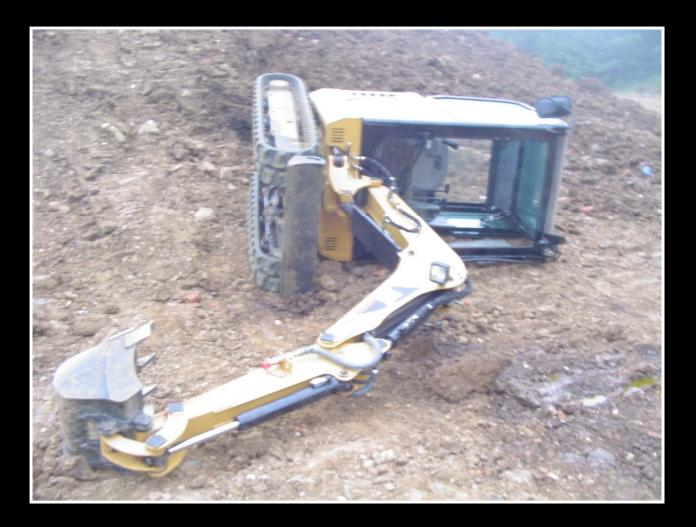
Operator was travelling down a grade when it overturned. Operator was not wearing his seatbelt and was thrown from seat trapping his leg and foot between the front corner post of the cab and the ground.
