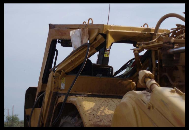
This machine was traveling on haul road and started skidding. The operator tried to correct for the skid when machine rolled over. Operator was wearing seatbelt and was not injured.
