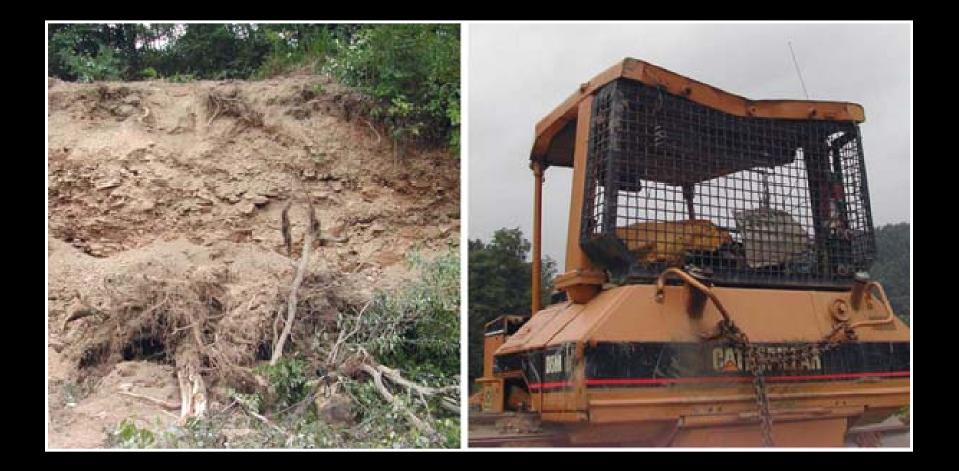
COAL MINE FATALITY - A 50-year old operator with 26 years of mining experience was fatally injured while operating a bulldozer. The operator was using the bulldozer to clear trees on top of a 24-foot high embankment to facilitate construction of a haul road. While he was pushing material toward the edge, the bulldozer traveled over the crest of the embankment, coming to rest on its side.
