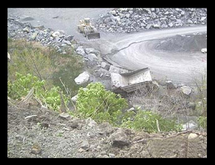
On April 25th, 2007, a 65 year old truck driver with 42 years of mining experience was fatally injured at a cement operation. The victim was operating a haul truck that veered off the roadway, climbed a berm, and fell over a high wall onto a bench below. The victim was not wearing a seat belt at the time of the accident and was ejected from the cab of the truck.
