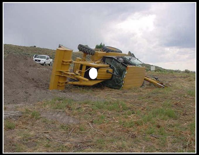
Operator was grading area when his rear tire went down to the left into some soft material and machine rolled on its side. Operator was not wearing his seatbelt at the time of the incident.
