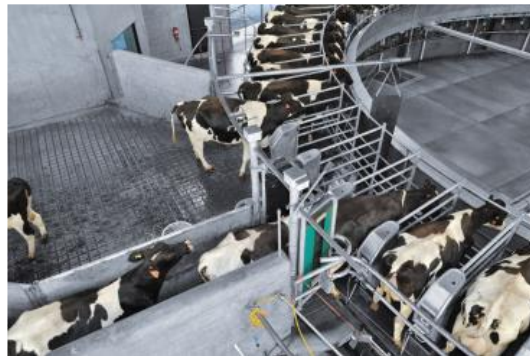
Rotary Stall - Any stall on a moving platform, which revolves around a central axis. These stalls may be either a herringbone (cows milked from inside) or parallel (cows milked from the outside).
